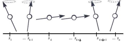
Fig. 5. Separating magnetization vectors into coordinate positions which are in the slice,  $S_{\text{in}}$ , and out,  $S_{\text{out}}$ .
