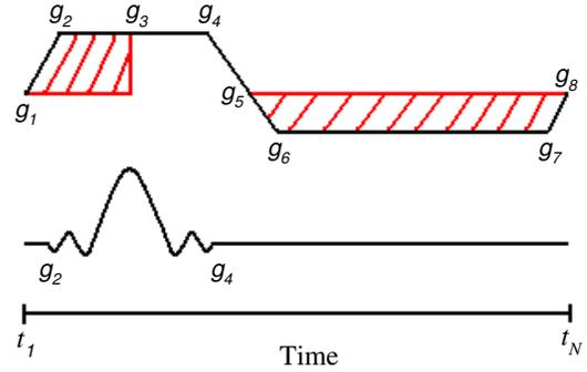
Fig. 7. The initial solution for the gradient function  $G(t)$  (top) and external magnetization  $b_y(t)$  (bottom).
