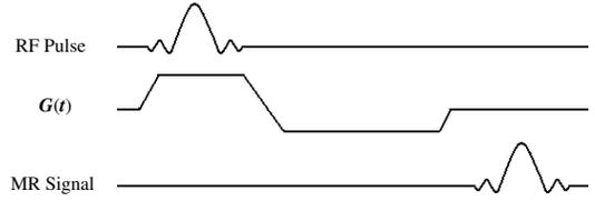
Fig. 1. A generic NMR slice select pulse imaging sequence.
