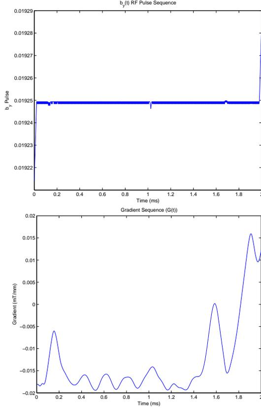
Fig. 13. External magnetization component  $b_y(t)$  and gradient sequence  $G(t)$  for the 15 slice results,  $b_x(t)$  is zero.
