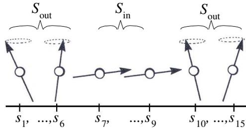
Fig. 8. The separation of coordinate positions  $s_i$  into  $S_{\text{in}}$  and  $S_{\text{out}}$  for 15 magnetization vectors.
