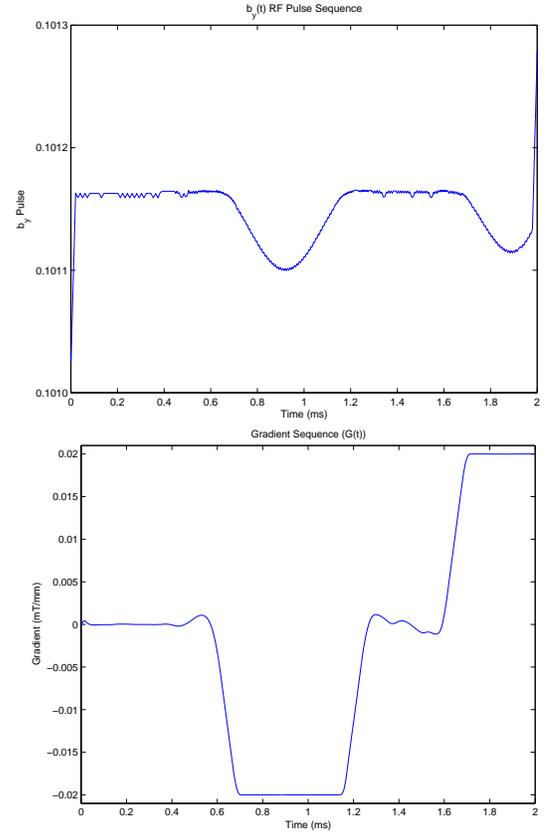
Fig. 14. External magnetization component  $b_y(t)$  and gradient sequence  $G(t)$  for the 15 slice penalty results,  $b_x(t)$  is zero.
