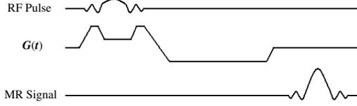
Fig. 2. The VERSE pulse imaging sequence.
