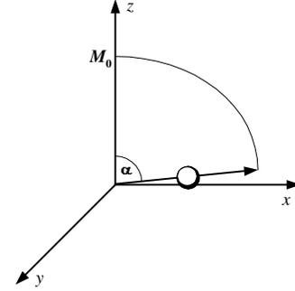
Fig. 6. The initial solution for magnetic moment vectors in  $S_{\text{in}}$  that have tipped into the transverse plane by an angle of  $\alpha$ .
